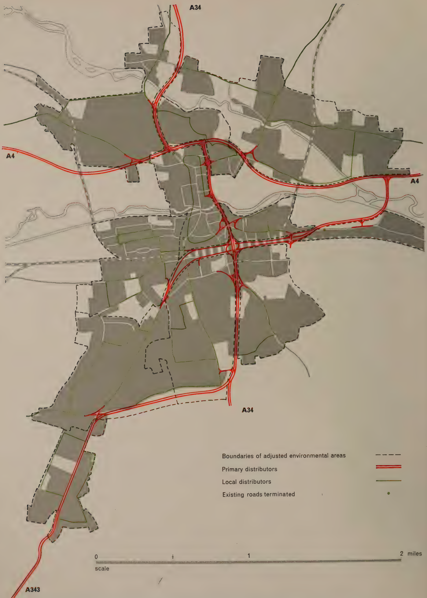
88 The proposed new primary network with local distributors and adjusted environmental areas.
